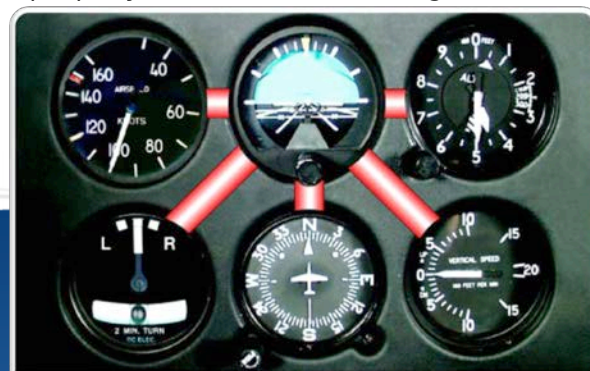
Figure 6-1. In most situations, the cross-check pattern includes the attitude indicator between the cross-check of each of the other instruments. A typical cross-check might proceed as follows: attitude indicator, altimeter, attitude indicator, vertical speed indicator
